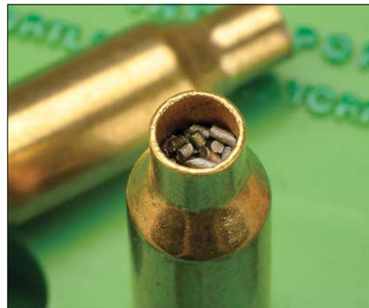
The only compressed load tried consisted of 36.0 grains of RL-15 over a Nosler spitzer resulting in a velocity of 3,986 fps and a .575-inch group at 100 yards.
