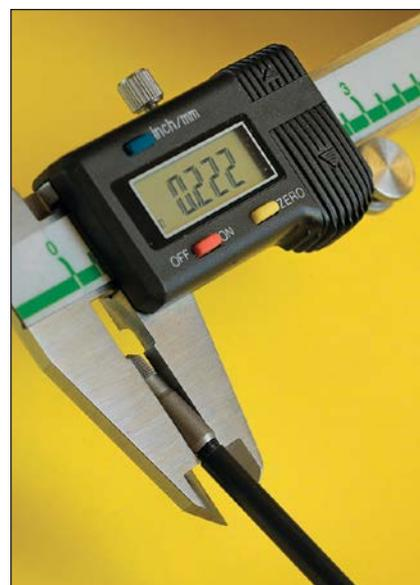
The case neck expander button on the Redding die used measured .222 inch, which provides reasonable neck tension to hold bullets in place when using the single-shot test rifle.
