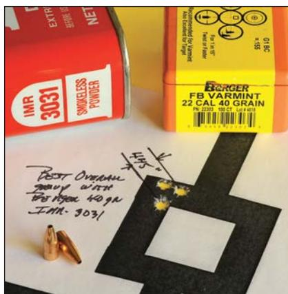
At .441 inch, this is the best group of the entire series and was shot with Berger 40-grain flatbase bullets over 32.0 grains of IMR-3031 for a velocity of 3,848 fps.
