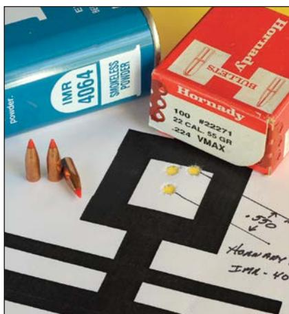
Hornady 55-grain V-MAX bullets over 32-grains of IMR-4064 resulted in this .550-inch, 100-yard group.
