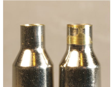
Case necks vary little in thickness. Uniforming them by trimming (right) resulted in no accuracy gains over a standard case (left).
