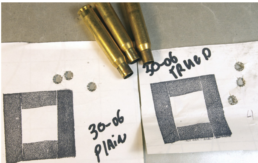
Handloads built on ordinary .30-06 cases and trued cases resulted in no significant accuracy difference.
