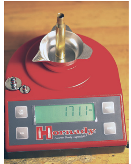
Segregating cases by weight ensures a batch of them has the same internal dimensions. Today's cases are so uniform, however, that weighing them is a waste of time for hunters.
