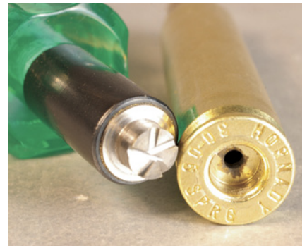
A primer pocket cutting tool scraped some brass off the face of primer pockets in Hornady .30-06 cases.
