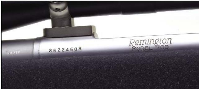
*The Remington stainless Model 700 action was originally chambered for the .30-06 but easily accommodates the longer 7mm STW.*
